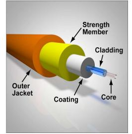
No light escapes until it comes to the end of the fiber, unless the fiber is bent sharply or stretched.
