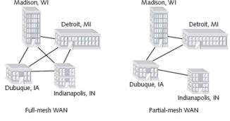
Mesh WANs are the most fault-tolerant type of WAN configuration because they provide multiple routes for data to follow between any two points.
