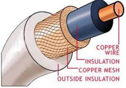
• The next layers, collectively referred to as the shield, keep electrical impulses and radio transmissions out.
